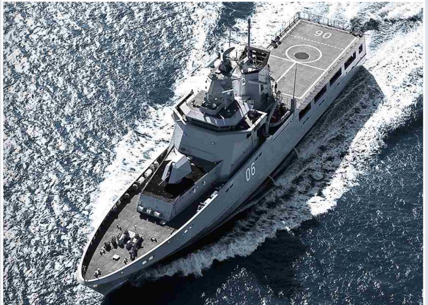
Above. Images of the original 1993 OPC design are hard to come by, but the winning contender for the 2018 OPV, the Lurssen OPV80, gives a good idea of the concept. At 80-metre is the same length as the OPC design, but with a Displacement 26% greater (Image: Lurssen).
